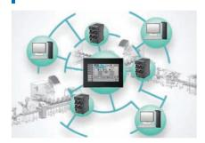
Ethernet communications allow you to access all controllers on a production line and the PC from one HMI, which is impossible with serial communications.
